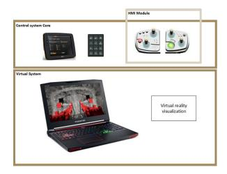
Main dimensions (Digital Driller™ one module) TV screen (not included) 15" touch screen 430 display 1 210 HDMI Laptop included 535 450 LAN Protection case(s) approx. weight: 25 kg Simulator approx. weight 20 kg
