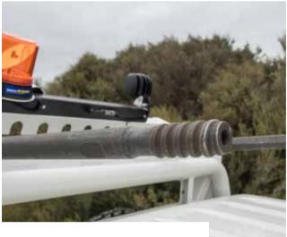
The rods are double-clamped and strapped down to ensure secure transport.
