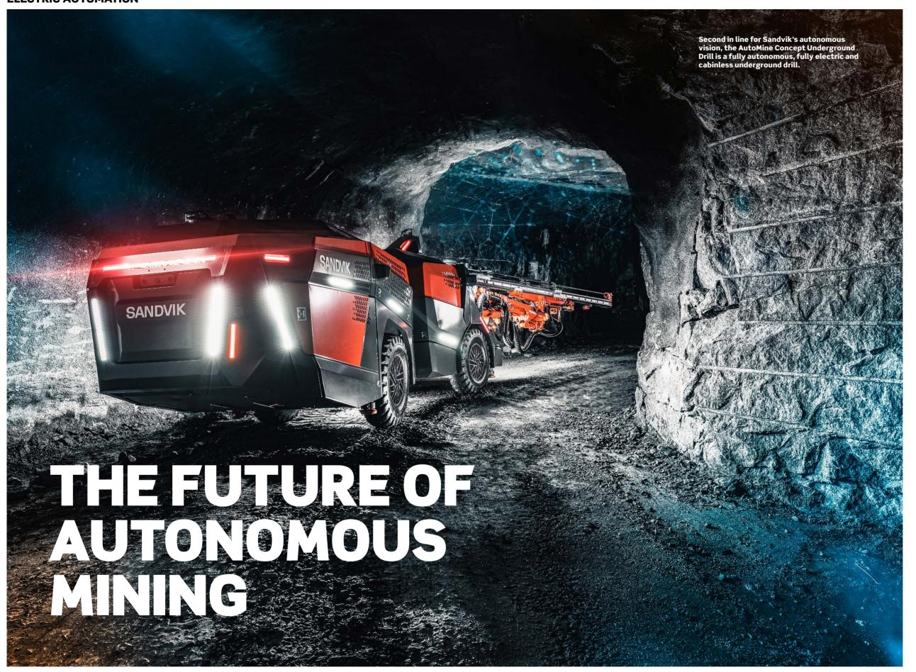
The AutoMine Concept Underground Drill is the next generation of autonomous drilling. The cabinless batteryelectric machine is the company's next evolutionary step in automation.
