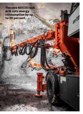
and reel structure, individually adjustable hose support structure, automatic greasing of joints as well as easily adjustable and changeable slide pieces provide excellent maintainability.
