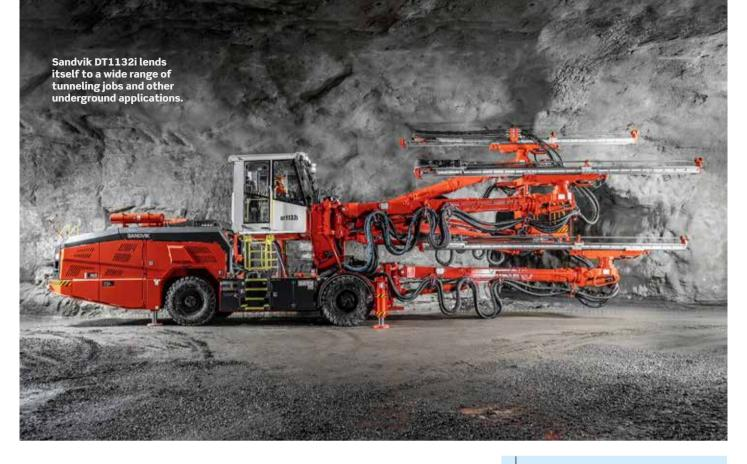
**THE CURRENT DEVELOPMENT** trends in tunnel drilling call for equipment to be as versatile as possible. A single drill rig should preferably be capable of face drilling and bolt hole drilling as well as longhole drilling jobs. Another key requirement is the ability to collect data while drilling, analyze it onboard or in the office and utilize it for applications such as quality control purposes, 3D profiling and water loss measurements.
