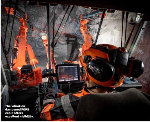
connectivity capabilities with two automation levels, the standard Gold package for operatorcontrolled boom positioning and the optional Platinum package for full face drilling automatics. Both options feature powerful control and measurement systems for torque-based drilling, drilling depth and angle, drill bit location, drill plan visualization as well as rig navigation – in other words, more accurate drilling.
