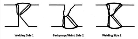
Fig.2: Welding Side 1 / Backgouge and Grind Side 2 / Welding Side 2
