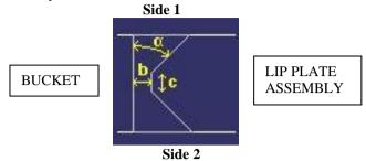
Fig. 1. Double-bevel butt weld preparation
