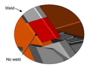
This method is to ensure that the bar does not add internal stresses to the Cast Corner which may lead to fatigue cracking.
