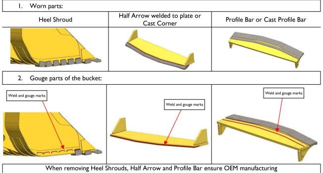
When removing Heel Shrouds, Half Arrow and Profile Bar ensure OEM manufacturing procedures, local site safety procedures, and welding procedures are followed.
