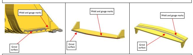
4. Perform NDT (Non-Destructive Testing) on the gouged area of the bucket to ensure no cracking exists. If cracks are found regrind to remove entire cracks and reweld according to PWP0001 and relevant OEM welding procedure:
