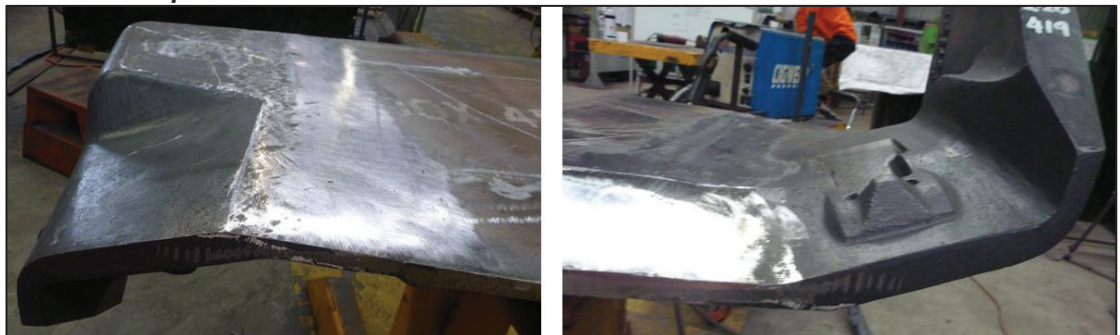
Figure 42 cast corner weld visual inspection
