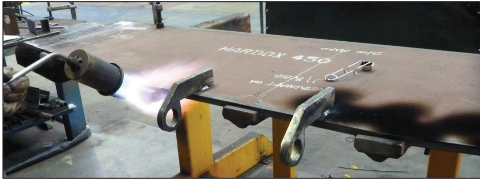
Figure 31 Pre-heating at 1G position
