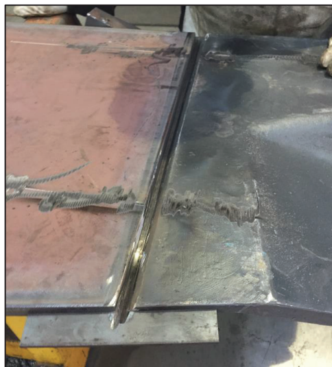
Figure 15 Back Grind weld
