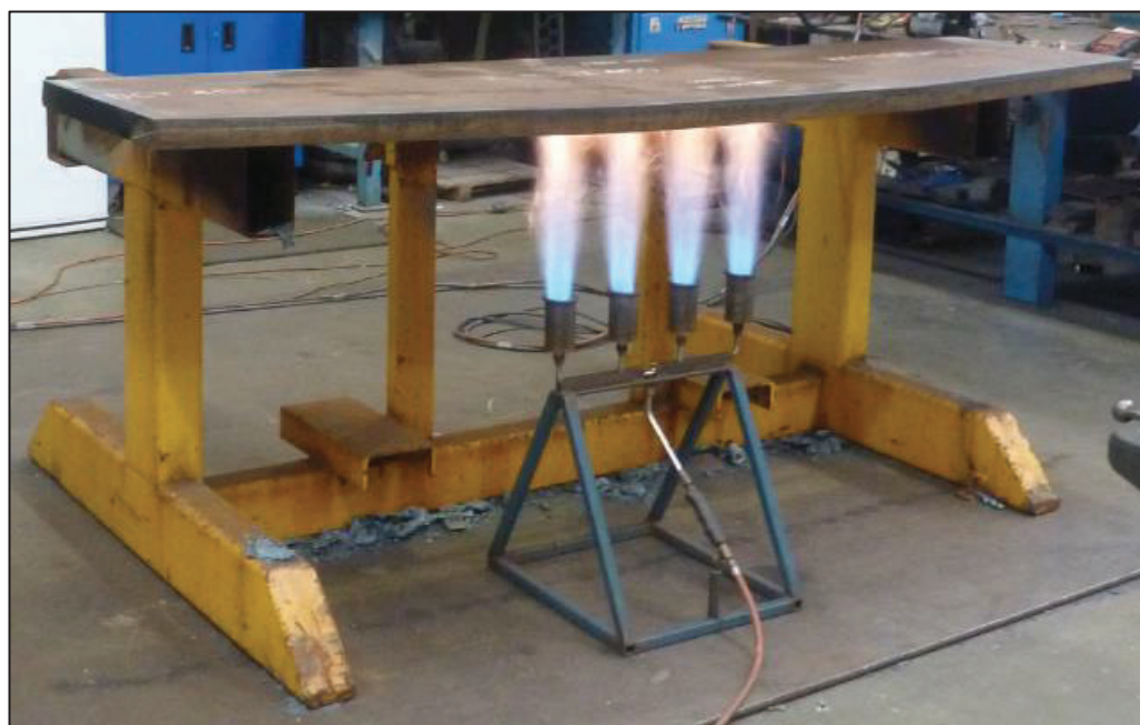
Figure 3 Preheating Hardox plate
