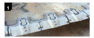
**METHOD 1**: Ensure bucket is empty and clean. Pressure wash the shrouds thoroughly, especially at the locking system cavity area to clear all debris. Ensure all nearby personnel are at a safe distance during pressure-wash and all necessary PPE is used.
