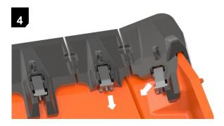
Remove lock assembly once shroud has been cut. Wash the locking system cavity to remove any remaining fines. The shroud should now be able to be removed from the lip.
