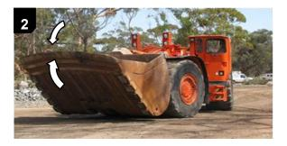
**METHOD 2:** If shroud still cannot be removed using method-1, drive the Loader to a level and flat location, a safe distance away from any personnel. Use machine hydraulics to bounce the empty bucket upwards and downwards without hitting the ground to dislodge the fines from the pin assembly. Do not perform loading with the bucket if any shroud become dislodged as it will damage the lip.
