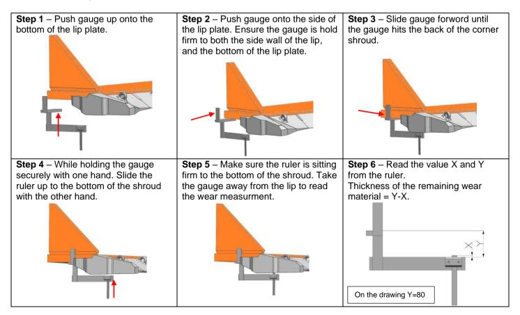
First measurement has to be taken, when Half Arrow are first welded onto the lip. This procedure has to be used along with "Half Arrow Corner Wear Gauge – Measuring spreadsheet".
