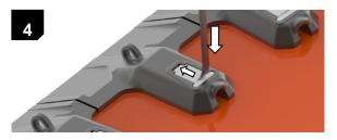
Insert a pry bar into the slot between the Spacer and the Pin Block. Push the Pin Block forward to break the seal between them.
