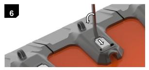
Lever back the Pin Block until it hits the rear of the cavity.
