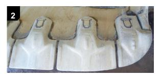
Ensure bucket is empty and clean. Pressure wash the shrouds thoroughly, especially at the Cap screw and Pin Assembly cavity area to clear all debris. Ensure all nearby personals are at a safe distance during pressure-wash and all necessary PPE is used. Follow Sandvik recommended Safe Work Procedure SWP0002 during shroud removal process.
