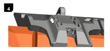
Rotate the Hexagonal Bolt head Anticlockwise direction (Using a Torque Wrench 19mm socket) to push the Pin Assembly in 15mm from the lip.
