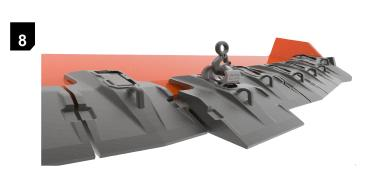
Slide the shroud off lip while fully supported by the MAKO  $^{\text{TM}}$  shroud lifting device.
