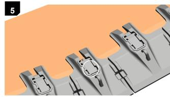
Tighten the bolt three (3) turns in Clockwise direction to release lock tabs from cavity. Ensure locking system is forward enough to release locking tabs.
