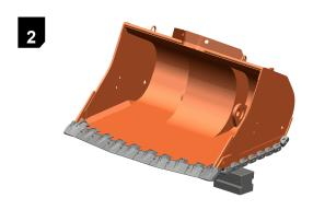
Position the bucket using a bucket holding device or bucket stands. Ensure bucket is empty and clean. Pressure wash the shrouds thoroughly, especially at the Pin Assembly and Bolt Plug cavity area to clear all debris. Ensure all nearby personals are at a safe distance during pressure-wash and all necessary PPE is used. Follow Sandvik recommended Safe Work Procedure SWP0008 during shroud removal process.
