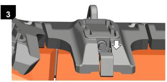
Remove the Bolt Plug from the rear of the Hexagonal Bolt head. Be aware to wear appropriate hand protection.
