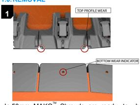
In 50mm MAKO $^{\text{TM}}$  Shrouds are ready to be changed when wear indicator become visible or reached in one or both of the (top and Bottom).
