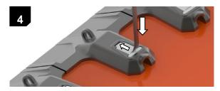
Insert a pry bar into the slot between the Spacer and the Pin Block. Push the Pin Block forward to break the seal between them.
