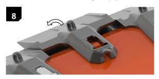
The shroud can now be removed from the Lip. Following removal, wash down the lip using a power washer, ensuring the lip profile is clean and ready for installation of the replacement shroud.
