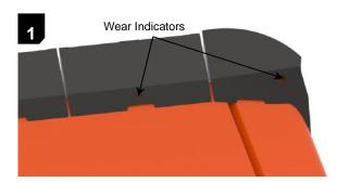
BLUE POINTER™ II Series Lip Shrouds are ready to be changed when the wear indicators become visible at the base of the shrouds as shown.
