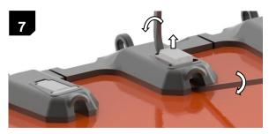
Lever out the Pin Block using two pry bars.
