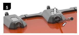
Insert pry bar into the cavity under the Spacer and pry Spacer up and remove it from the Shroud.
