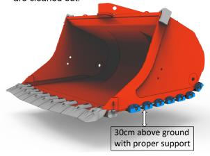
Important: Ensure that the bucket is properly supported with Cat stands or similar supports before installation.
