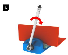
Torque the bolt to 400 ft/lb (540 Nm).
