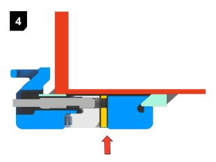
Pull the bolt back so that the nut is against the adapter. Place the spacer between the shroud and the back of the nut through the gap that is created.
