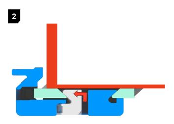
Apply anti-seize to nut. Insert nut into the heel shroud cavity from the bottom with the chamfer of the nut facing the bolt hole of the shroud. Then pull the nut towards the bolt hole of the shroud as shown above.
