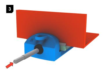
Apply anti-seize to bolt. Insert bolt through the shroud and adapter bolt holes. Thread the bolt through the nut. Tighten the bolt with a ¾ inch socket wrench.
