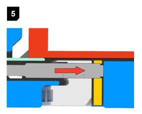
While holding up the nut and spacer in place, tighten the bolt so that it passes through the nut and the spacer.
