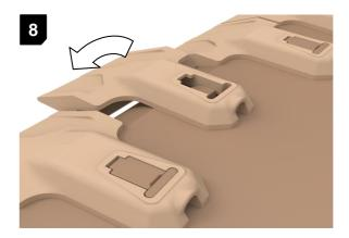
The shroud can now be removed from the Lip. Following removal wash down the lip using a power-washer, ensuring the lip profile is clean and ready for installation of the replacement shroud.
