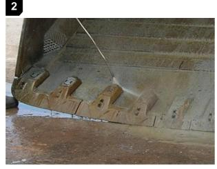
To begin the removal process a power washer should be used to remove any build up of fines from around the Cap Screw and Pin Assembly Areas.
