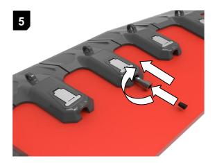
Insert Cap Screw through the arch at the rear of Shroud, then through the hole in the Spacer until it engages the thread in the Locking Pin. Turn clockwise to tighten, using a torque wrench with a 5/8" socket to achieve **250ft.lb** (339Nm).
