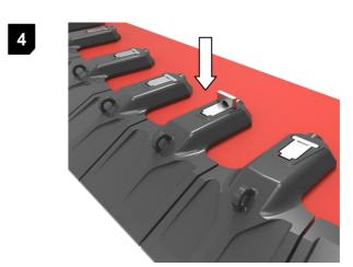
Insert Spacer downward into the remaining cavity at the rear of locking pin.
