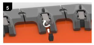
Access the hexagonal Bolt head at the rear of shroud. Turn clockwise to tighten, using a torque wrench with a 19 mm (or ¾") socket to achieve 700 Nm (516 ft.lb). During tightening, tap the shrouds at the front-top edge using a well-dressed copper hammer to assist parts to align correctly.
