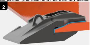
With the use of a mechanical aid, raise the shroud into a position to slide the rear of the shroud up and over the Boss and push home, ensuring the highlighted surfaces are in contact with the corresponding faces on the lip. Ensure the front edge of the tooth are inline.
