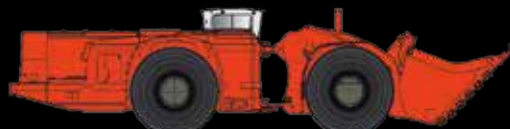
Sandvik LH621 Capacity 21 000 kg Tunnel size 5.5 x 5.5 m
