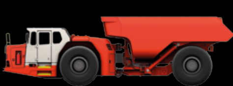
Sandvik TH551i Capacity 51 000 kg Tunnel size 5 x 5 m
