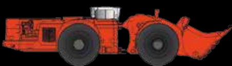
Sandvik LH517 Capacity 17 200 kg Tunnel size 5 x 5 m
