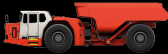
Sandvik TH663i Capacity 63 000 kg Tunnel size 6 x 6 m
