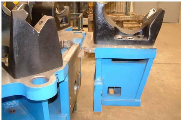
1. Clean all contact surfaces. Oil bolts, nuts, wedge and slotwedge. Hook the segment on to the head as shown.
