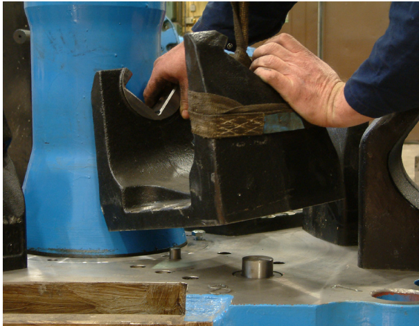
1. Remove the inner saddles from position 1 and 2. Use the tool combination on page 8
