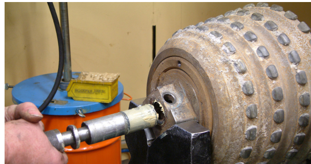
4. Remove the conical plugs (7008-9257) from the seal retainers. Use proper allen key wrench (7008-9447).
