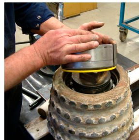
7. Install the two seal halves (7008-9110) in both the retainer ring and the cutter shell. Important! Follow the mounting instructions from the seal manufacturer carefully. Instructions can be obtained from your local Sandvik representative.
