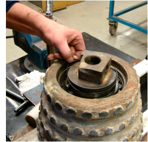
4. Remove the two seal halves from both the seal retainer and the cutter shell. Remove the O-ring 7008-9604 (under the seal retainer).
