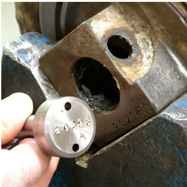
Cutter serial number is found on the shaft end of the narrow part of the cutter and on the ball plug retainer.
