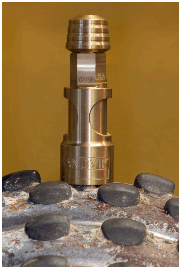
Use measuring gauge 7008-9631 to measure the button wear on any individual button. The gauge measures the percentage of the protrusion left on each button.
