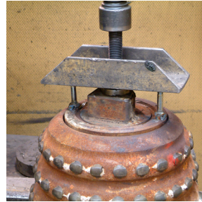
3. Make a puller tool by using two bolts, nuts and a small U-beam. Tack weld the two bolts to the retainer ring. Remove the retainer ring by tightening the nuts and tapping the retainer ring with a hammer. The retainer ring can be reused if it is not damaged.
