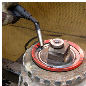
10. Mount the protection ring 7008-9113 and weld four joints 90° apart. Use MIG welding. Recommended welding wire Ø 1,2 mm OK AUT-ROD 12,51 or similar.
