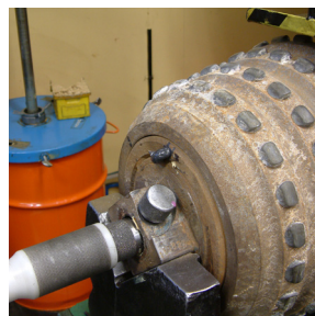
11. Re-grease the cutter according to the regreasing instruction. This completes the seal change.
