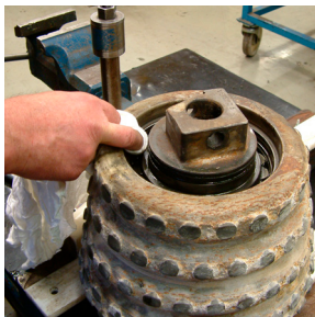
5. Clean the snap ring groove, the O-ring groove and the seal seat carefully. Ensure that the seal seat is in good condition. If not, file the marks and nicks. Make sure no muck or dirt comes in to the bearing system.
