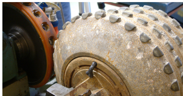
6. Start pumping until grease comes out through one of the relief holes. Clean the thread and mount the plug. Put some Loctite222 on the thread before tightening. Use the allen key wrench.
