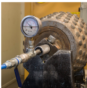
9. Pressure test to make sure the cutter seals are not leaking.
