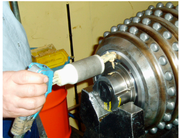
2. Attach a grease pump and start pumping.
