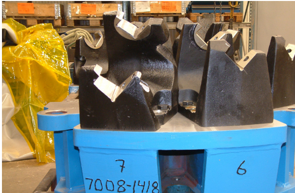
1. The positions are marked on the side of the head frame. If there are two position marks, the upper one refers to the position nearest the head centre.
