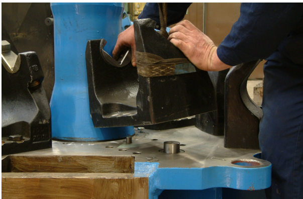
10. Mount the saddles in position 1 and 2 (see picture on page 8). The head assembly is now complete.
