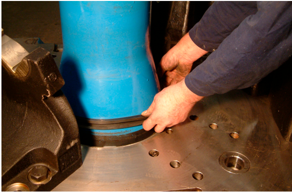
6. Clean the seal seat. Slide the V-ring over the top of the stem and push it into position. Note. Do not use the V-ring in reaming head CRH3 and CRH4.
