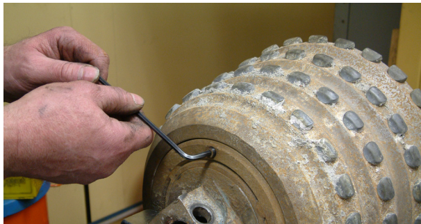
3. Pressure test to make sure the cutter seals are not leaking.
