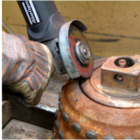
1. Cut the four welding joints on the sea retainer. Use a small cutting disc. Remove protection ring 7008-9113.
