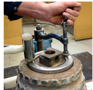
8. Mount the O-rings 7008-9604 (on the journal). Note. Lubricate the O-ring carefully with oil before installation. Mount the retainer ring carefully. E.g use a hammer and clamp for smooth mounting. Mount the snap ring 7008-9111. Note! Always use new O-rings and snap ring.
