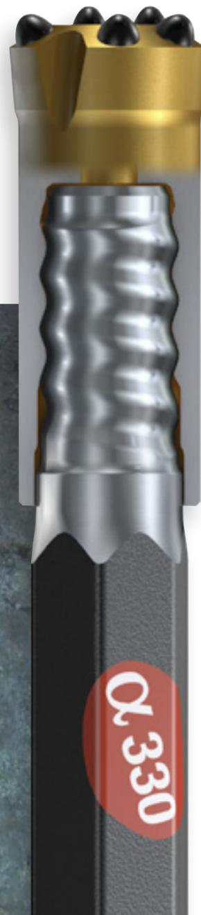
A snug interface at this crucial point at the rear of the connection greatly improves the rigidity of the joint. The bit skirt covers the thread completely in the Alpha 330 connection, no part of the thread itself is exposed to sandblasting, reducing the risk of corrosion-fatigue.
