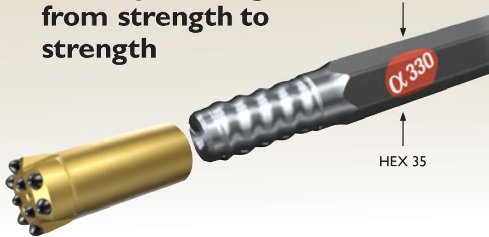
The new short thread design on the hexagonal rods in the tool system result in a rigid, integrated power pack drill string with superior resistance to bending stresses, improved bit guidance and perfect energy transfer. The sturdy thread is well guided inside the bit skirt, offering high precision in collaring – even in complex rock formations and against uneven surfaces.
