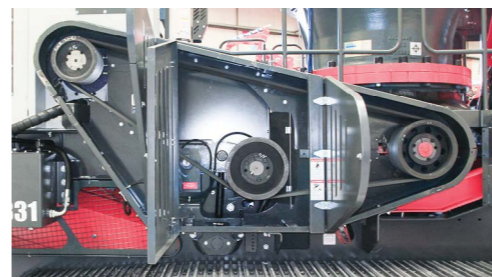
Direct drive for maximum fuel efficiency
