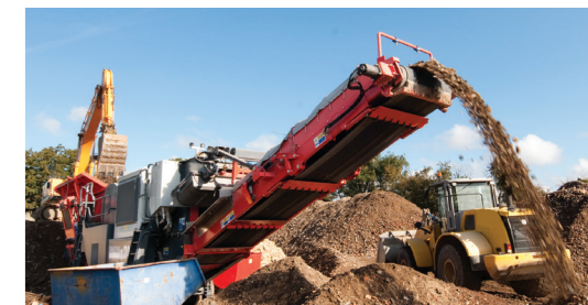
Extended main conveyor for massive stockpiling
