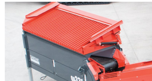
Hopper complete with hydraulic tipping grid
