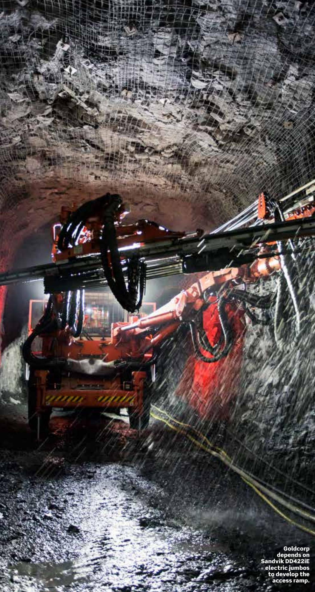
Goldcorp depends on Sandvik DD422iE electric jumbos to develop the access ramp.
