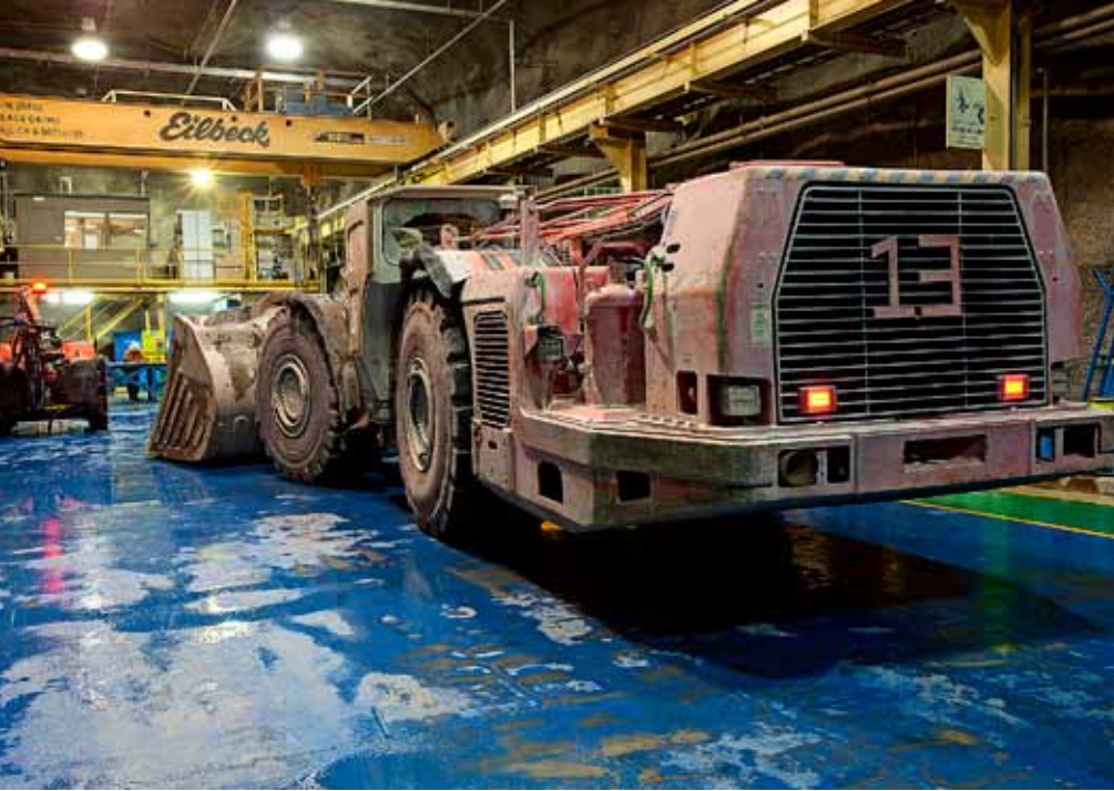
Six Sandvik LHDs have been fitted with the AutoMine loading system at Northparkes.
